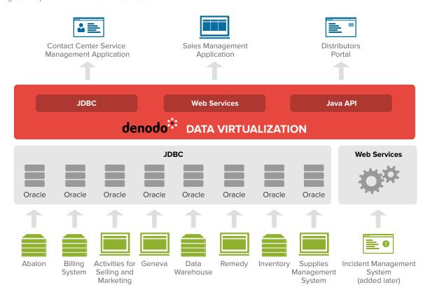
The Denodo platform was used to connect source systems that included Oracle databases containing customer data related to billing, subscriptions using JDBC and to the Incident management system using web services. This source data was combined within Denodo to create derived views or data services that were published to three major applications:
